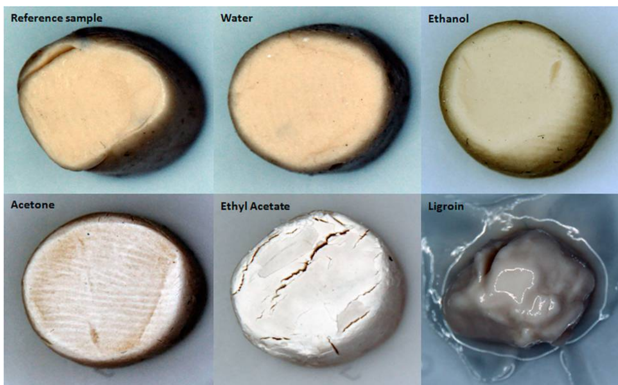
Figure 10 Solubility test, mock-up samples after one hour of immersion of Plastiline ® in several solvents. The reference sample was not immersed in any solvent. Photo credits: C2RMF.
