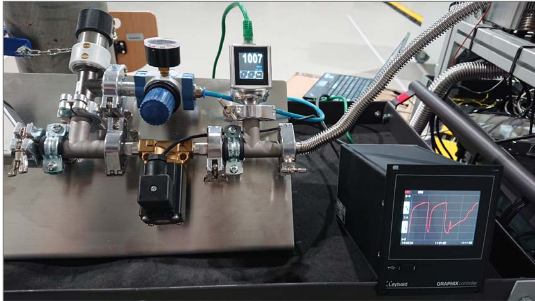
Mechanical and electrical fuse for overpressure protection
