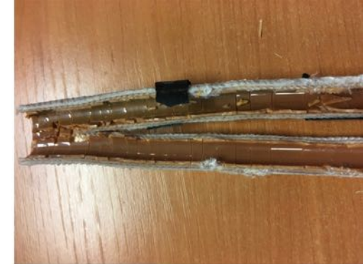
Exuding water along the hose (1 drop/sec)
