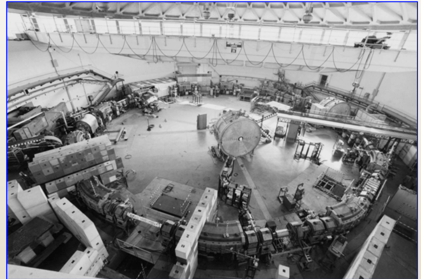
LNF ADONE (big ADA) electron-positron storage ring 1.5 GeV per beam, C = 105 m (1969-1993)
