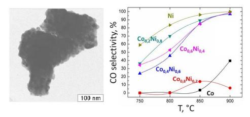
Figure 1: TEM image of the Nd<sub>1.3</sub>Ca<sub>0.7</sub>Co<sub>0.4</sub>Ni<sub>0.6</sub>O<sub>4</sub> reduction product after POM test (left) and the dependence of CO selectivity vs temperature for Nd<sub>2-y</sub>Ca<sub>y</sub>Co<sub>1-x</sub>Ni<sub>x</sub>O<sub>4</sub>-based catalysts with various Co/Ni ratio (right).
