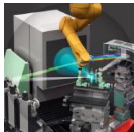
Figure 1. Schematic representation of the combined time-resolved X-ray methodologies at the FXE instrument.
