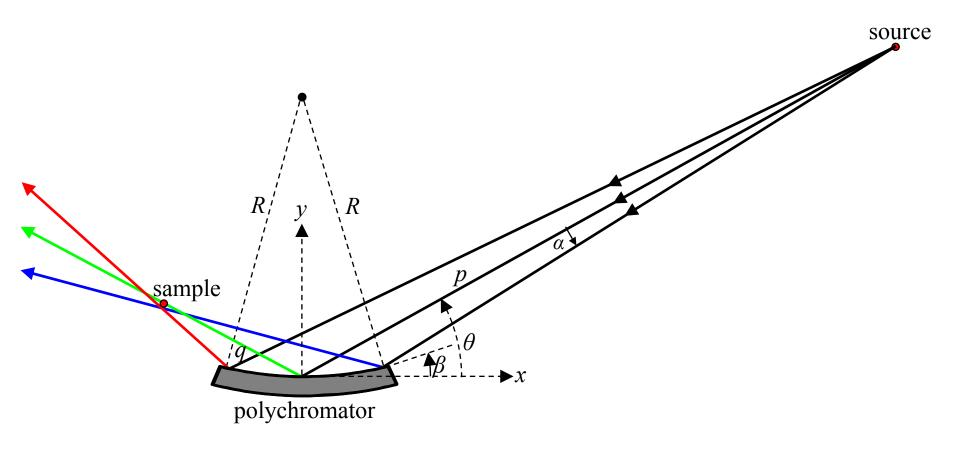
We find that the diffracted rays do not all meet at one point.
