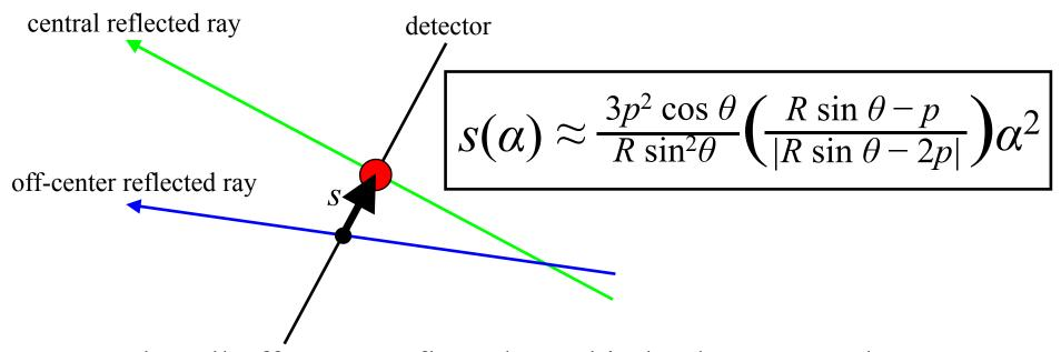
Note that all off-center reflected rays hit the detector on the same side of the central reflected ray!
