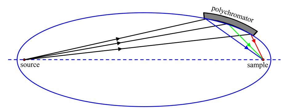
Specified elliptical bends can be approximated by cylindrical bends, which are easier to perform but introduce aberrations.
