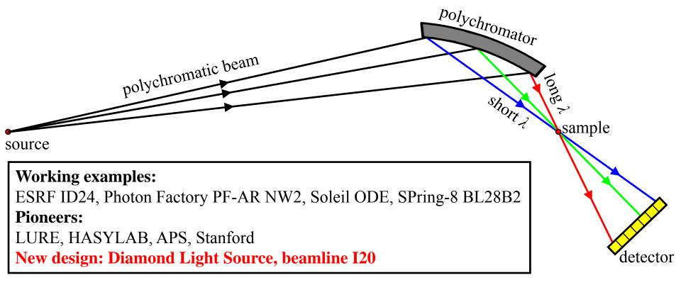
→ an X-ray absorption spectrum can be taken in a short time, without any scanning required.
