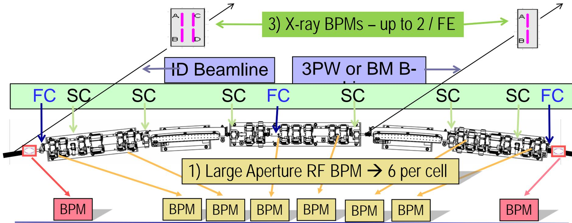
2) Small Aperture RF BPMs → 2 or 3 per Cell; Button Assembly on a Stand or ID Chamber
