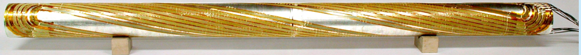
Picture of a helical dipole magnet coil
