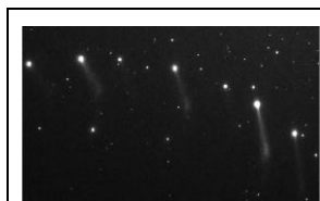
Figure 2 Typical Laue patterns for a probe volume containing a single crystal (a) many small well-crystallized grains (b) several grains with small or large orientation gradients (c).
