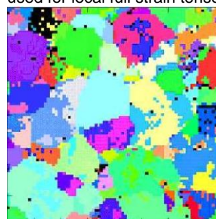
Figure 3 2D Orientation map from CdTe polycrystal with sample lateral steps of 5 \mu\text{m} .
