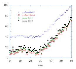
Now we want to determine from this data the moment at which the data points start to increase. This can be done by fitting the straight parts to linear functions and determining the intercept. The result is shown in the following figure:
