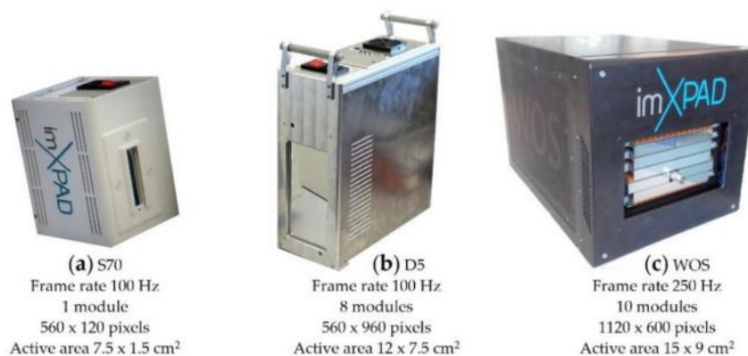
Figure 3. The ImXpad detectors available at the D2AM beamline: (a) the S70, (b) the D5, and (c) the WOS (wide-angle X-ray scattering (WAXS) Open for small-angle X-ray scattering (SAXS)).
