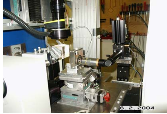
Fig.7 The set-up for alignment and calibration of high pressure experiments on the MAR345 area detector.
