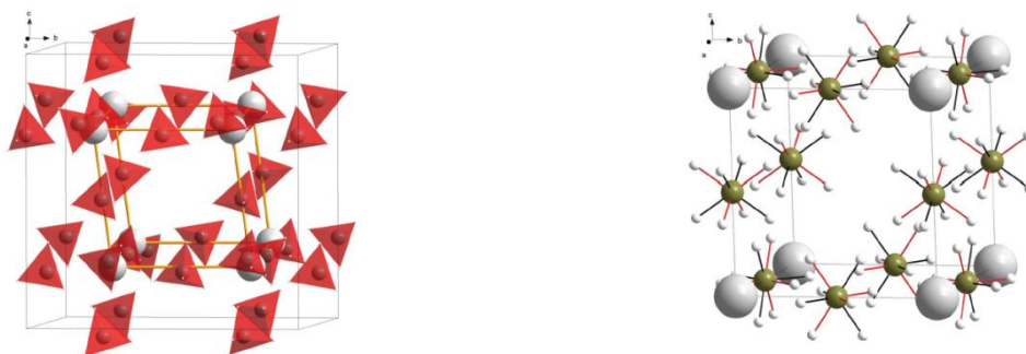
Figure 2: Unit cell for two different RE(BH 4 ) 3 polymorphs: \alpha -RE(BH 4 ) 3 (left) and \beta -RE(BH 4 ) 3 (right) as seen by SR-PXD, with RE atoms shown as light grey spheres. Note the disordered structure [18] ( Pm-3m , a \sim 5.5 \text{ \AA} ) on the right which becomes ordered ( Fm-3c , a \sim 11 \text{ \AA} ) when neutron diffraction is used instead [6].
