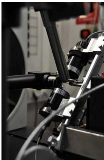
Figure III.7 Combined XRD+Raman+UV spectroscopy set-up
