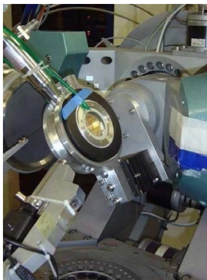
Figure III.6 Low temperature – Helium cryostat – Single crystal diffraction
