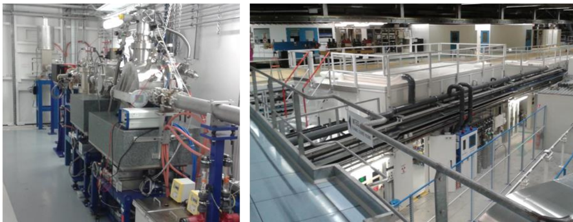
Figure 6. (Left) New BM31 optics enclosure and optical components. (Right) New hutches as seen from the bridge linking the Central Building with the machine control room
