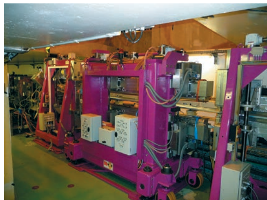
Fig. 160: The new 2.5 m-long helical undulator, installed on ID32, produces circular polarisation rather than only horizontal plane polarisation like most undulators.
